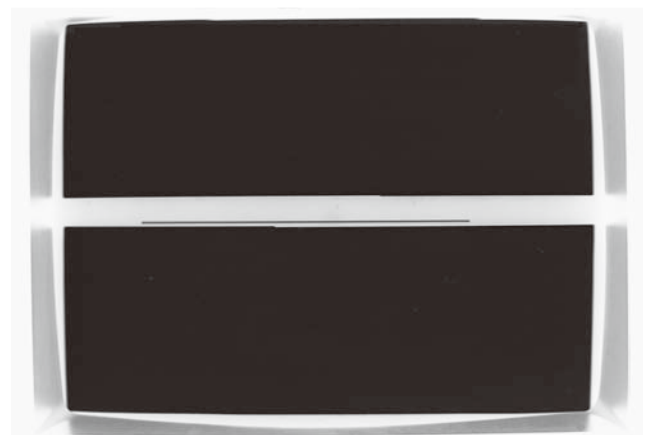
Photo 4: One-line measurement window in the vertical blanking interval
